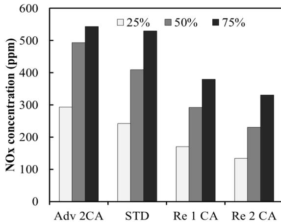
**Fig.10 Effects of different injection timing on NO**
