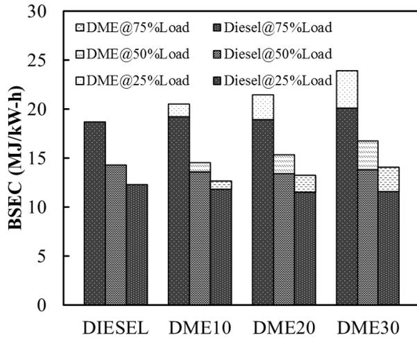
**Fig.3 Effects of different DME additions on brake specific energy consumption**
