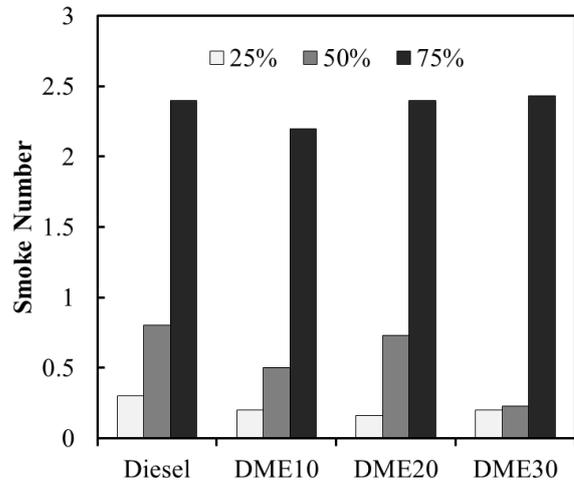
**Fig.5 Effects of different DME additions on smoke number**
