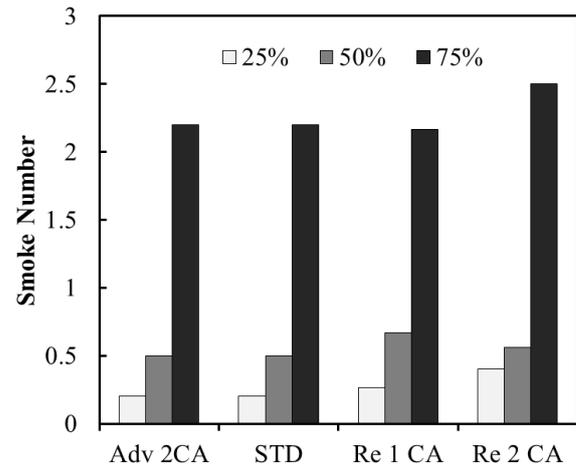
**Fig.12 Effects of different injection timing on SN**
