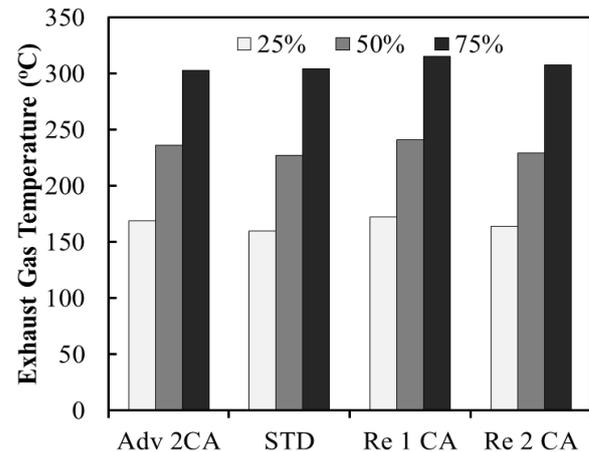
**Fig.13 Effects of different injection timing on exhaust gas temperature**
