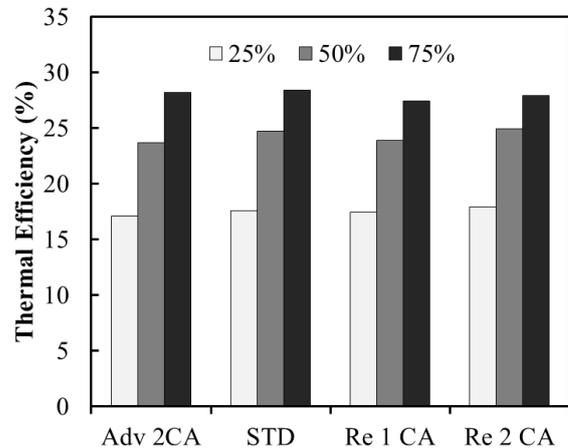
**Fig.9 Effects of different injection timing on Thermal efficiency**
