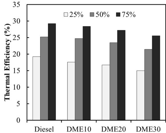
**Fig.4 Effects of different DME additions on thermal efficiency**
