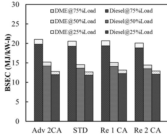
**Fig.8 Effects of different injection timing on BSEC**
