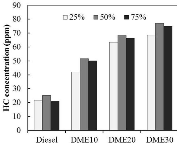
**Fig.7 Effects of different DME additions on HC concentration**
