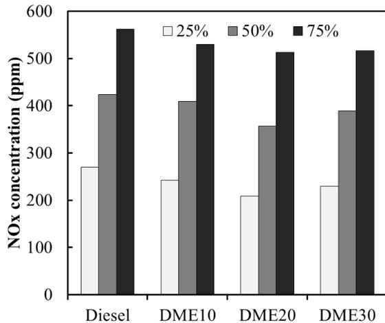
**Fig.6 Effects of different DME additions on NO concentration**
