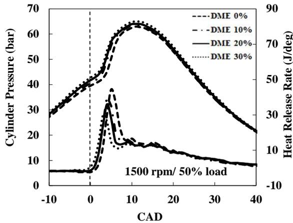
**Fig.2 Effects of different DME addition on In-cylinder pressure and HRR profiles**
