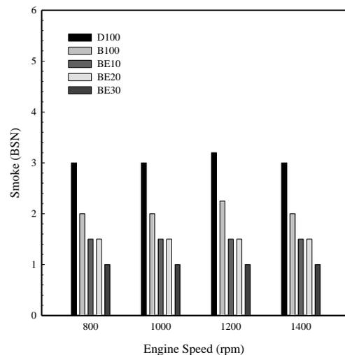
**Fig. 10** Relationship between black smoke and engine speed
