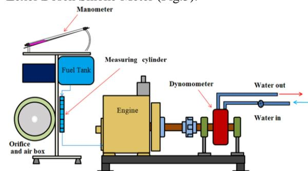
**Fig. 4** Experimental apparatus for testing the engine performance.
