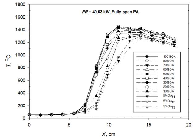
Fig. 6. Effect of  $OA$  on temperature profiles at medium  $FR = 40.6$  kW.
