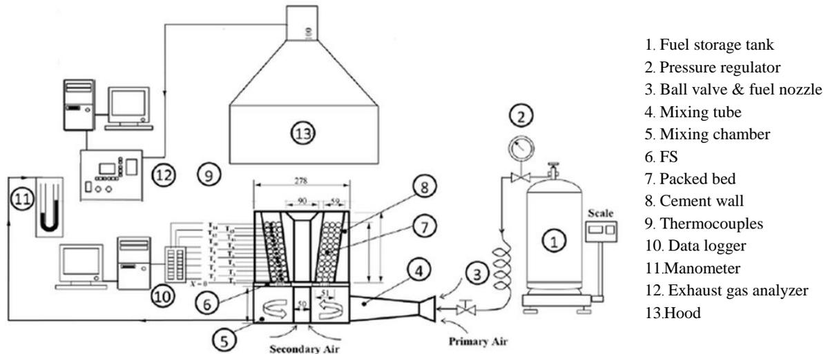
Fig. 3. Schematic diagram of the experimental set up.
