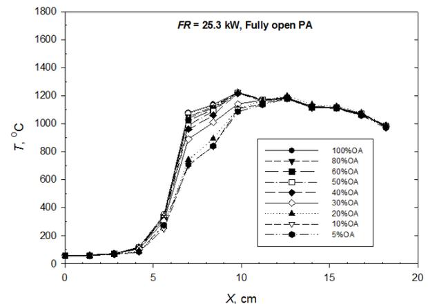
Fig. 7. Effect of  $OA$  on temperature profiles at low  $FR = 25.3$  kW.
