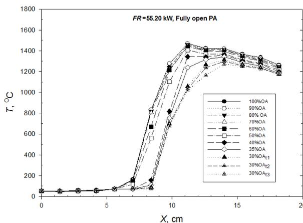
Fig.5. Effect of  $OA$  on temperature profiles at high  $FR = 55.2$  kW.
