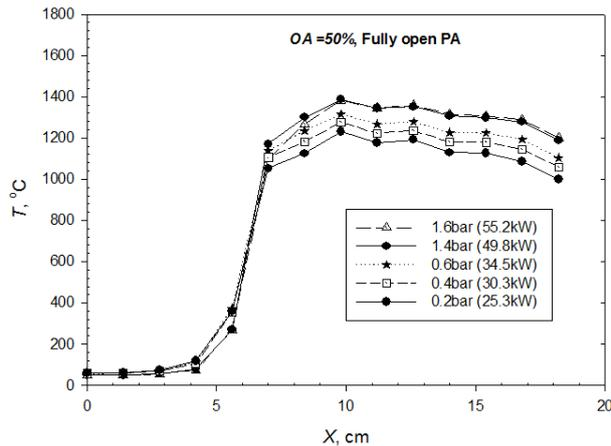
Fig.8 Effect of LPG inlet pressure on temperature profiles in the packed bed.
