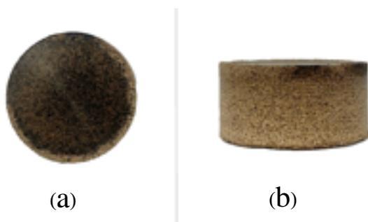
Fig. 4 Photos of the example biocoke prepared from rubberwood sawdust by using used coffee ground as a binder: (a) top view and (b) side view
