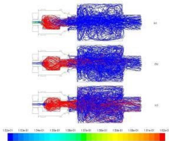
Fig. 11 Mass fraction of char particle trajectory (case 1); (a) 37.50-112.5, (b) 165.0-240.0, (c) 362.5-500.0  $\mu\text{m}$
