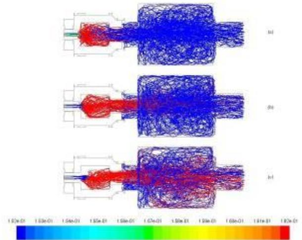
Fig. 12 Mass fraction of char particle trajectory (case 2); (a) 37.50-112.5, (b) 165.0-240.0, (c) 362.5-500.0  $\mu\text{m}$
