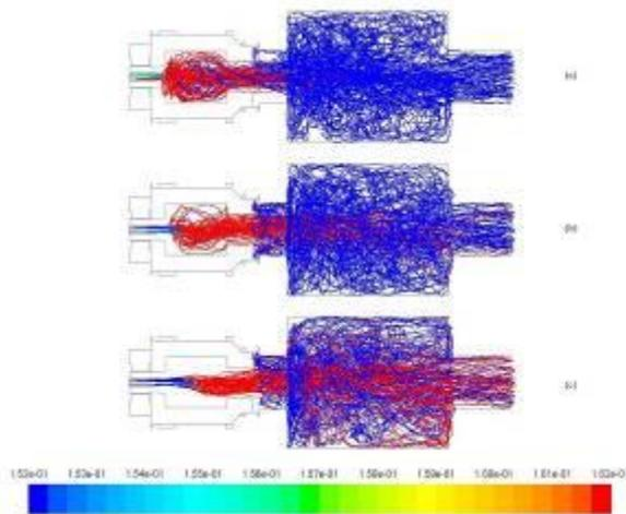
Fig. 18 Mass fraction of char particle trajectory (case 5); (a) 37.50-112.5, (b) 165.0-240.0, (c) 362.5-500.0  $\mu\text{m}$
