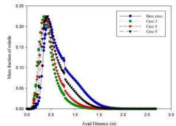
Fig. 19 Axial mass fraction of volatile of base case, case 3, case 4 and case 5
