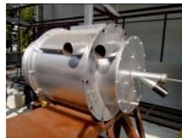
(a) Photograph of pulverized biomass burner
