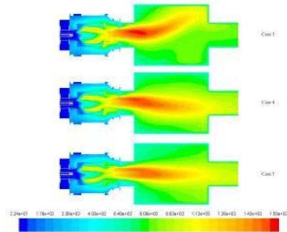
Fig. 14 Temperature distributions of case 3, case 4 and case 5 along the axial symmetry cross-section
