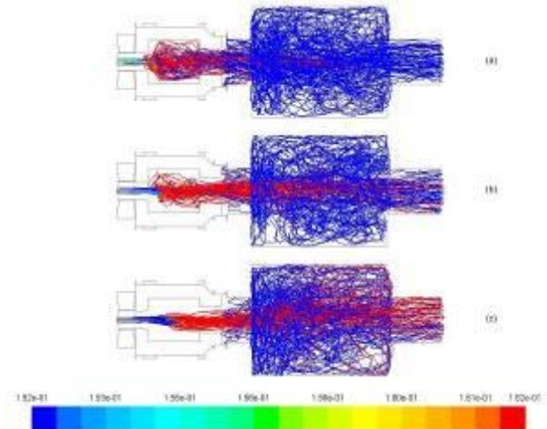
Fig. 8 Mass fraction of char particle trajectory (base case); (a) 37.50-112.5, (b) 165.0-240.0, (c) 362.5-500.0  $\mu\text{m}$
