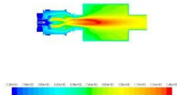
Fig. 7 Base case temperature distributions along the axial symmetry cross-section
