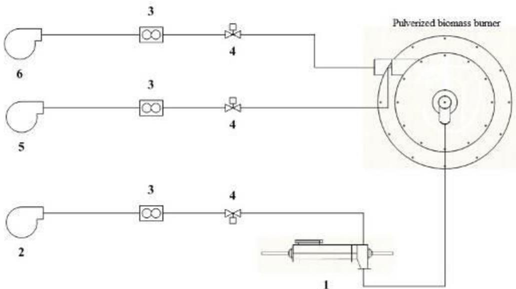
(b) Schematic diagram pulverized biomass burner of air system
