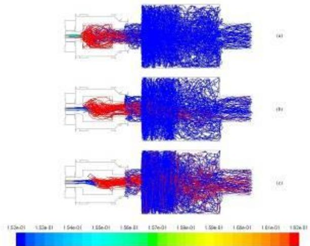
Fig. 17 Mass fraction of char particle trajectory (case 4); (a) 37.50-112.5, (b) 165.0-240.0, (c) 362.5-500.0  $\mu\text{m}$
