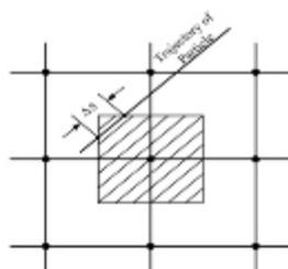
Fig. 4 Trajectory of particle for Lagrangian's Method
