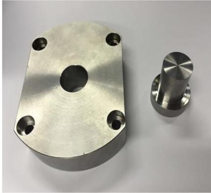
Fig.3 Mold for compressing bamboo powder sample
