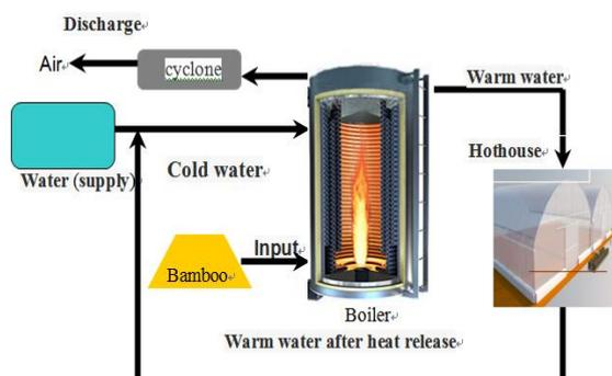
Fig.1 Concept of using wasted bamboo to warm a hothouse
