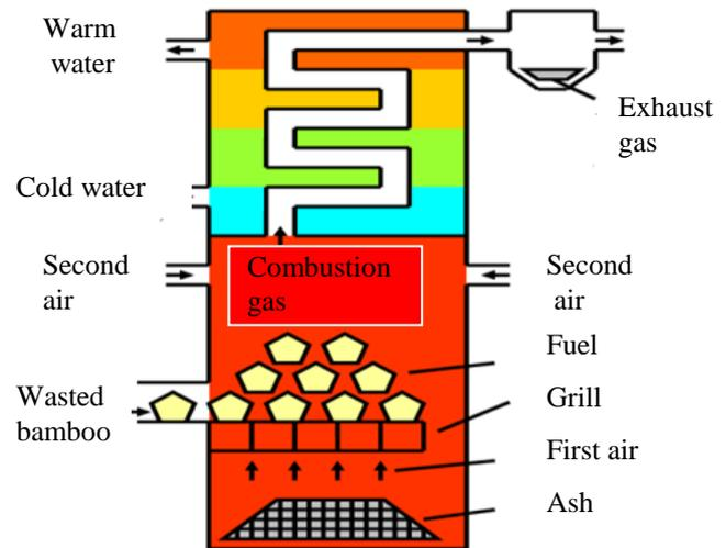
Fig.8 Concept model of the proposed boiler
