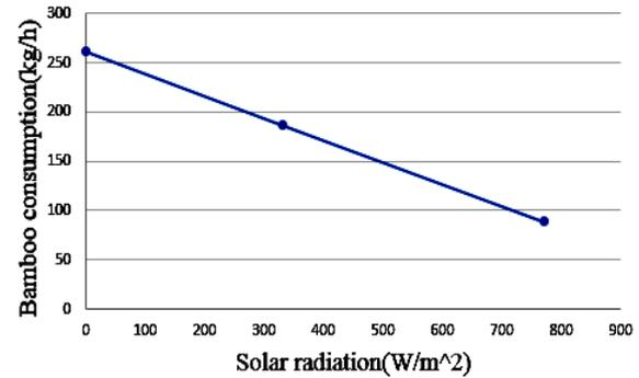
Fig.11 Relation between solar radiation and bamboo consumption
