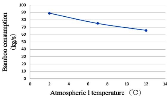
Fig.10. Relation between atmospheric temperature and bamboo consumption
