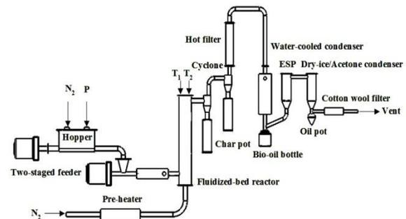
Fig. 1 Scheme of the laboratory plant for the sugarcane leaves and tops batch fast pyrolysis.
