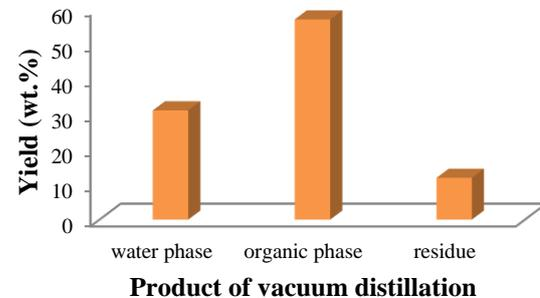
Fig. 4 Product yields of vacuum distillation from fast pyrolysis of sugarcane leaves and tops
