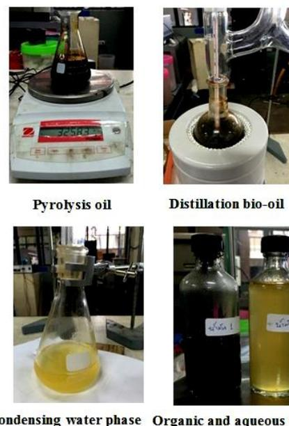
Fig. 5 Pyrolysis oil and products of vacuum distillation from fast pyrolysis of sugarcane leaves and tops.
