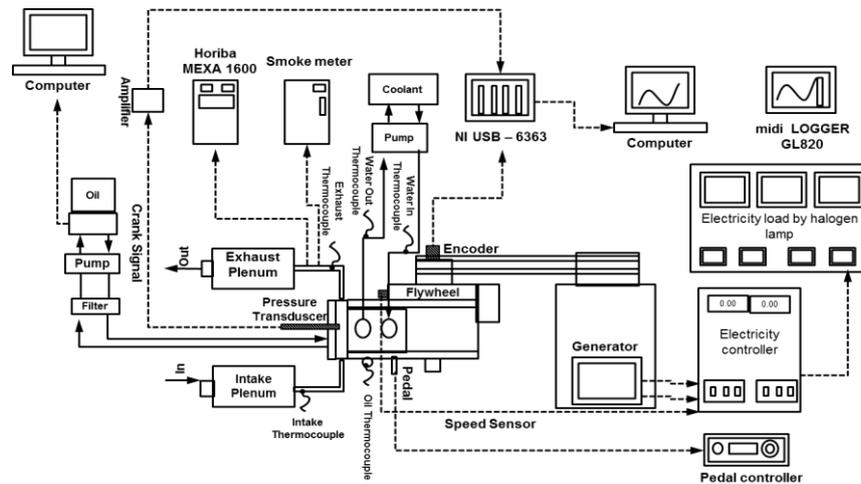
Fig. 1 The schematic diagram of the engine connected with the experimental apparatus.
