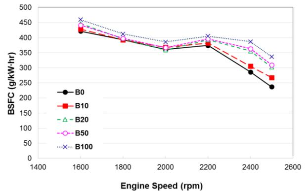
Fig. 4 Break specific fuel consumption when using H-FAME and its blends compared with diesel.
