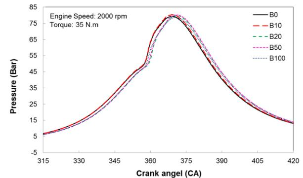
Fig.6 In-cylinder pressure of H-FAME blended fuels compared with pure diesel
