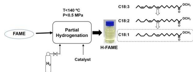
Fig. 2 H-FAME production from partial hydrogenation process
