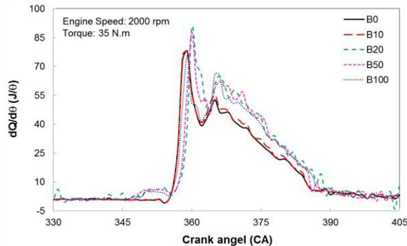
Fig. 7 Heat release rate of H-FAME blended fuels compared with pure diesel.
