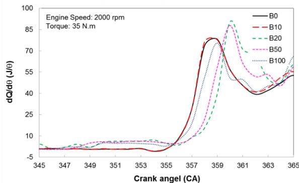
Fig. 8 The magnification of heat release rate to exhibit the start of the premixed combustion of each test fuel.
