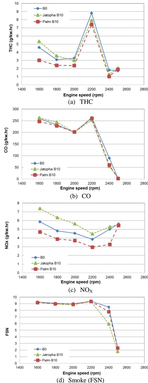
Fig. 5 Engine out exhaust emission when using B10 (jatropha and palm H-FAME) compared with B0 (a) THC (b) CO (c) NO<sub>x</sub> and (d) Smoke.
