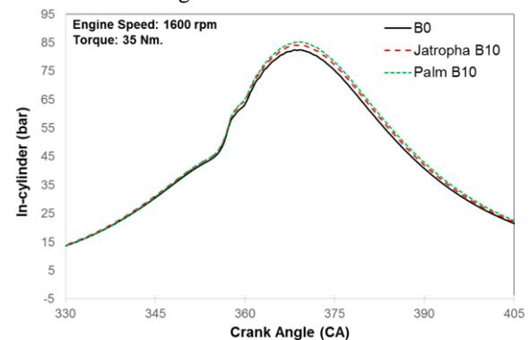
Fig. 6 In-cylinder pressure of B10 from jatropha and palm H-FAME compared with pure diesel
