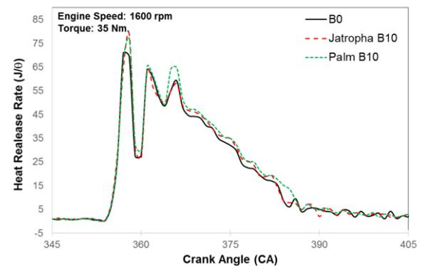
Fig. 7 Heat release rate of B10 from jatropha and palm H-FAME compared with pure diesel
