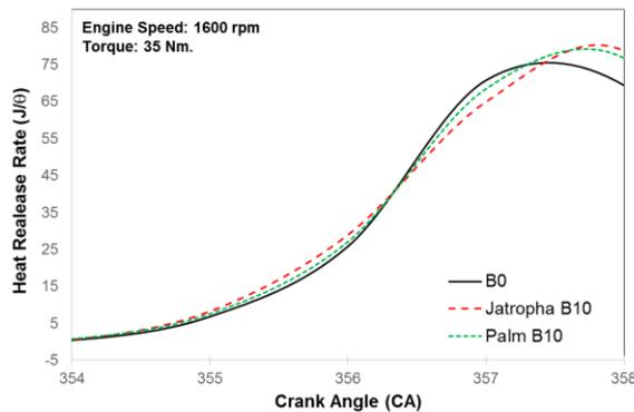
Fig. 8 The magnification of heat release rate of B10 from jatropa and palm H-FAME compared with pure diesel
