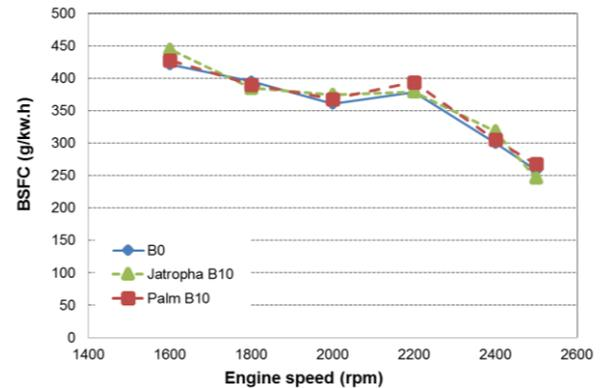
Fig. 4 Brake specific fuel consumption when using B10 (jatropha and palm H-FAME) compared with B0
