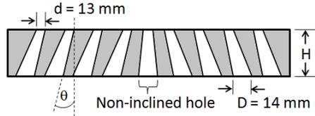
Fig. 3 The honeycomb plate with inclined holes ( $\theta$ )
