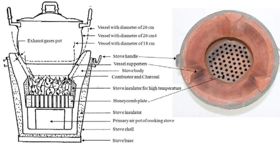
Fig. 1 A high efficiency cooking stove (HECS)
