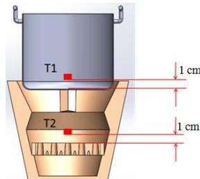
Fig. 4 The position of measured temperature in the present study
