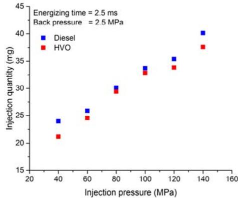
Fig. 8 Injection quantity and various injection pressure
