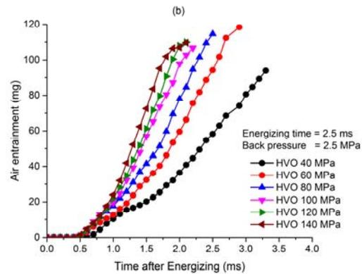
Fig. 9(b) Air entrainment of HVO and various injection pressure
