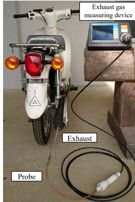
Fig. 8 Exhaust gas measuring device
