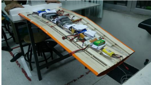
Figure 8. Characteristics of placing weight distribution on the wing.
