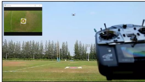
Fig. 8 The flight test of a quadrotor with wind speed 5 knot.
