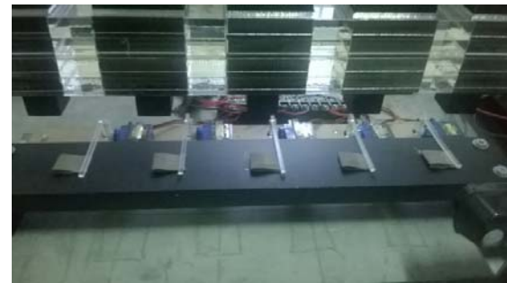
Fig. 15 Clamp the fabric samples by RC servo motors.
