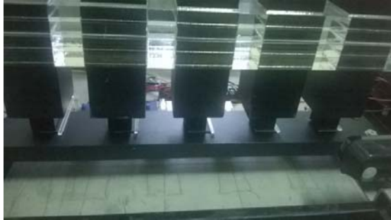
Fig. 16 Place the loads on the fabric samples.
