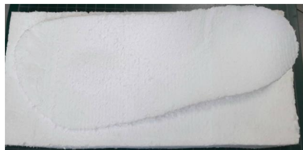
Fig.15 The customized insole was engraved by using the 3-milling head toolpath.
