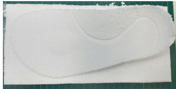
Fig.14 The customized insole was engraved by using the 1 milling head toolpath.
