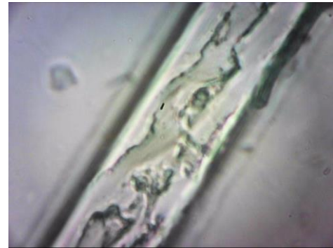
Fig. 11 The coarse surfaces on the channel walls of the new PDMS LOC.
