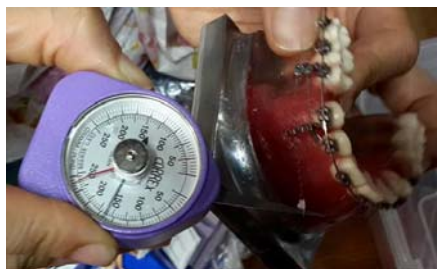
Fig. 2 Two Newton force measurement using tension gauge
