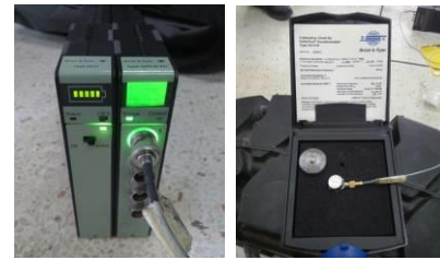
Fig.3 vertical acceleration measurement equipment
