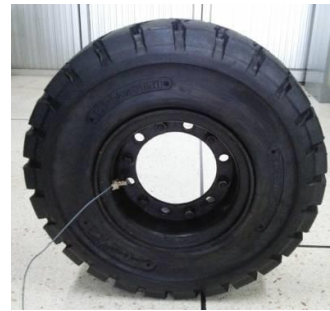
Fig.2 the position of accelerometer mounting
