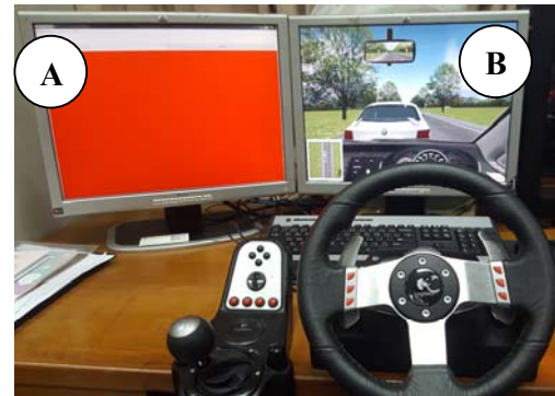
Fig. 2 CARNET Soft driving simulation (B) and Forward collision warning program (A).
