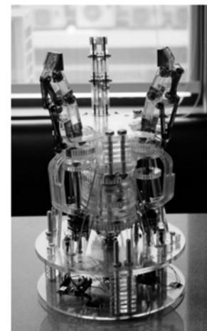
Fig.8 Three-finger robot hand after manufacturing process
