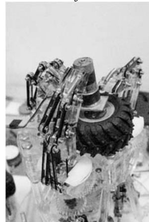
Fig.13 The result of grasping non symmetrical object
