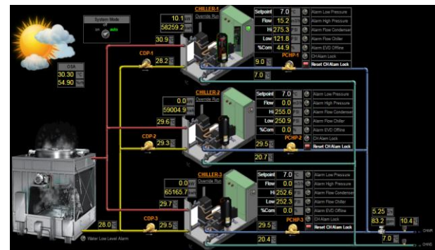
Fig. 6 Web-based monitoring of chiller system
