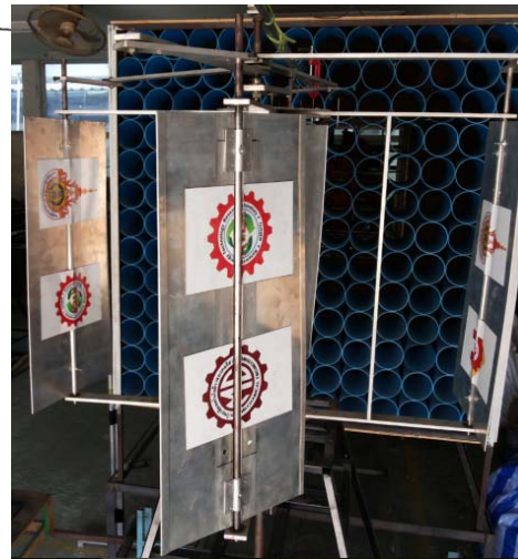
Fig. 3. Shows (b) components of four-bars linkage wind turbine and (a) photo of tested model
