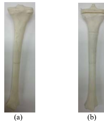
Fig. 11 Bone model: (a) Tibia bone and (b) Tibia bone inserted tibia component.
