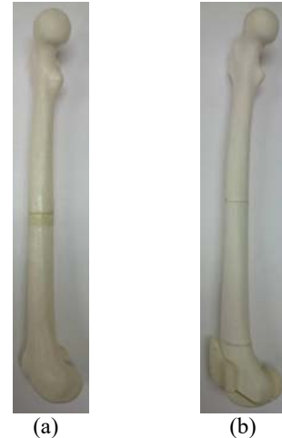
Fig. 10 Bone model: (a) Femoral bone and (b) Femoral bone inserted femoral component.
