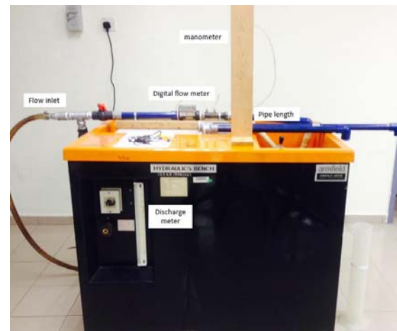
Figure 3 Experimental model for analysis the contaminant and fluid flow
