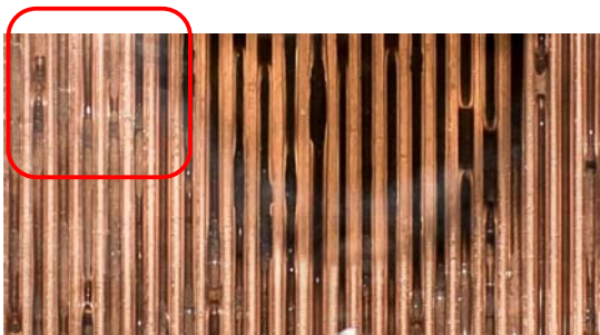
(d) Throat-annular flow with j_G = 3.31 m/s j_L = 0.417 m/s
