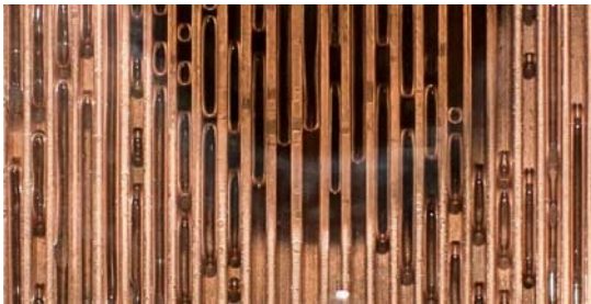
(b) Slug flow with j_G = 0.625 m/s j_L = 0.417 m/s
