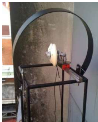
Fig. 2 The pyranometers and a shadow ring
