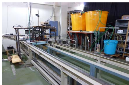
Fig. 4 Photograph of an experimental set-up with a stationary water tank and towing apparatus for Re = 10^2 - 10^3 .
