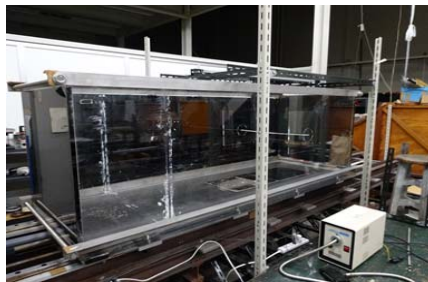
Fig. 3 Photograph of an experimental set-up with a towing water tank and stationary apparatus for Re = 10^1 - 10^2 .
