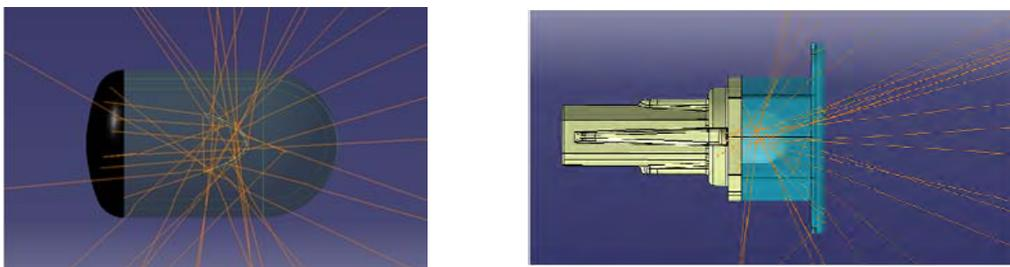
**Figure 3.** Ray tracing analysis for license plate lamp
