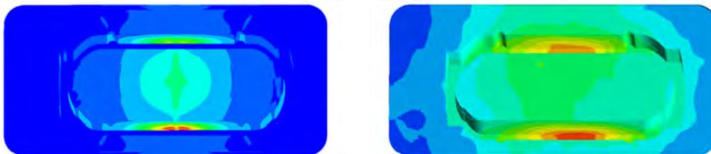
**Figure 15.** Comparison between hot spot area by ray tracing and FE thermal distribution on the covered lens
