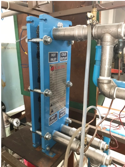
Fig. 3 KAUDY plate heat exchanger model M2 in the test rig
