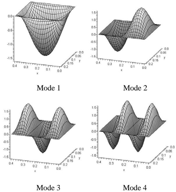
Figure 6. Vibration mode shapes of specimen No.2
