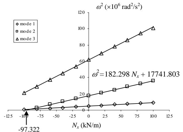
Figure 3. Plot of  $\omega^2$  and  $N_x$  of specimen No. 1
