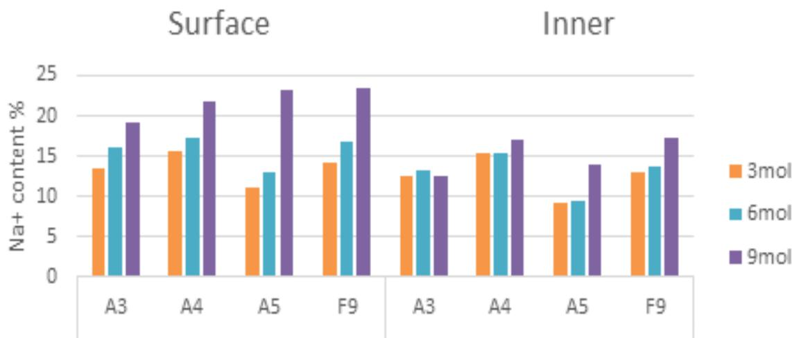
Figure 3. Na<sup>+</sup> content change after zeolite preparation
