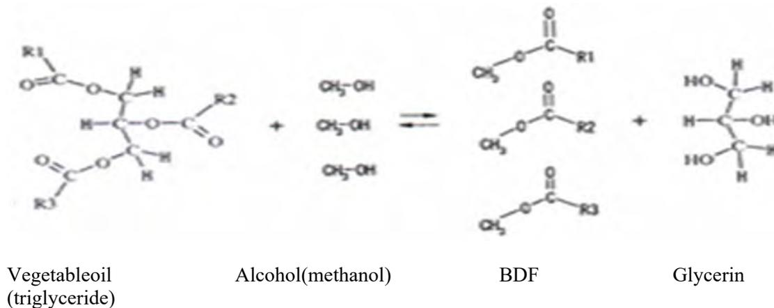
Figure 1. BDF synthesis principle
