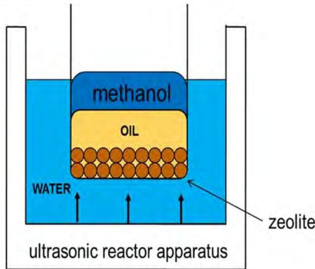
Figure 2. BDF synthesis by using batch method
