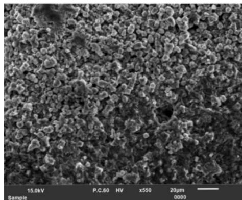
(b) SEM analysis result Figure 1. Shape of zeolite A5 and its SEM analysis.
