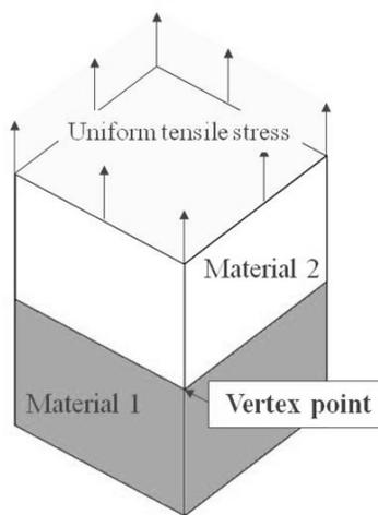
Fig. 2 Vertex point in three-dimensional bonded joints.
