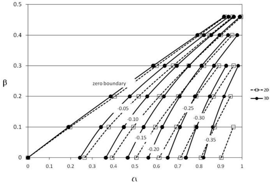
Fig. 6 The order of stress singularity on the Dundur's parameter plane  $\alpha - \beta$  for the vertex point in three-dimensional bonded joints.
