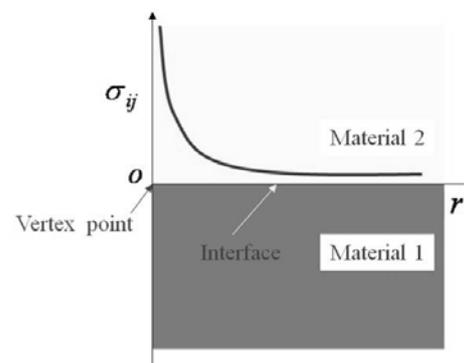
Fig. 1 Stress singularity at vertex point.
