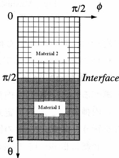
Fig. 3 Mesh model for FEM eigen analysis.
