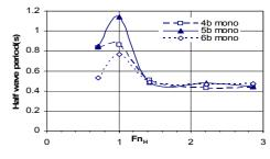
Fig.17 Half wave period of leading wave, H=0.2m
