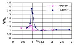
Fig.6 Resistance Ratio (5b monohull)
