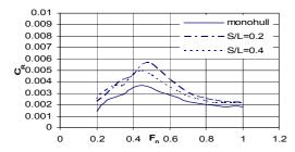
Fig.3 Residuary resistance coefficients (5b H=1.85m)
