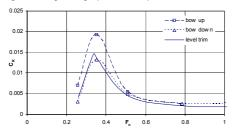
Fig.10 Residuary resistance coefficients (5S catamaran S/L=0.2 H=0.2m)
