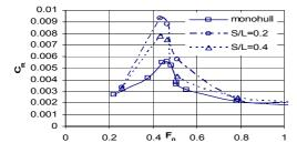
Fig.4 Residuary resistance coefficients (5b H=0.4m)
