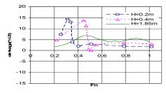
Fig.9 Running Sinkage (5b monohull)
