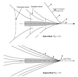
Fig.19 Sub-critical and supercritical wave patterns
