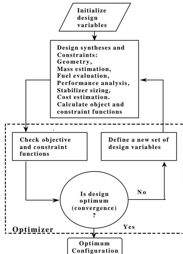
Figure 1 Basic algorithm of the MVO
