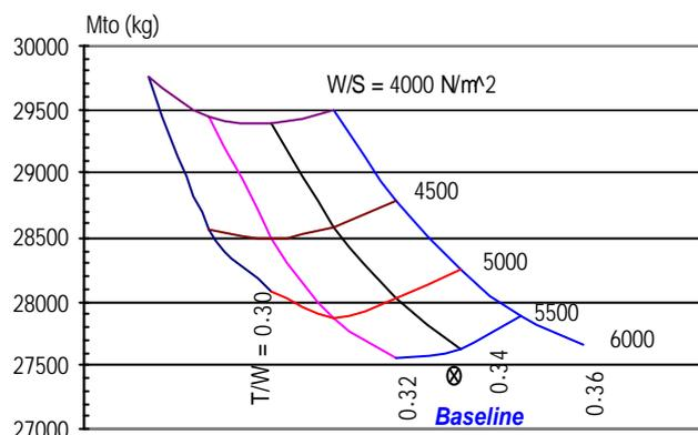
Figure 8 Effect of aircraft T/W and W/S on the takeoff mass of the baseline aircraft
