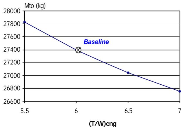
Figure 7 Effect of engine thrust to weight ratio
