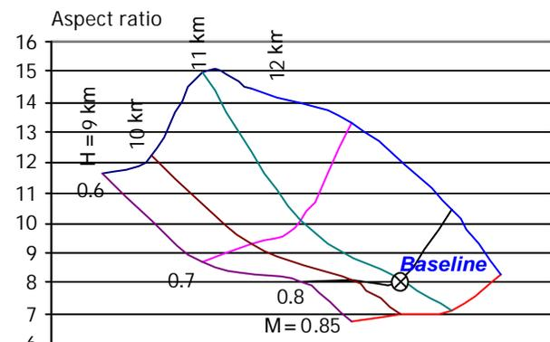
Figure 4 Variation of aspect ratio with cruise conditions
