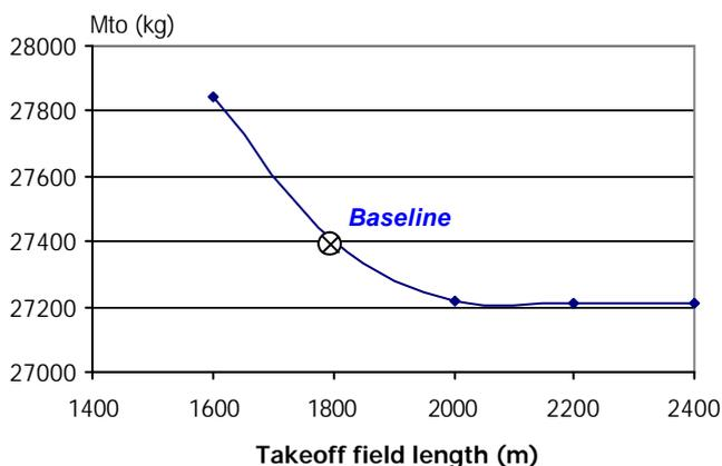
Figure 6 Effect of takeoff field length on the takeoff mass
