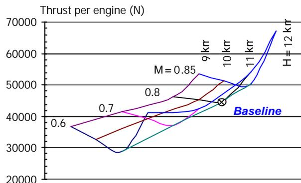
Figure 5 Variation of takeoff thrust with cruise conditions
