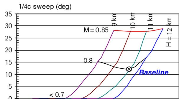
Figure 3 Variation of wing sweep with cruise conditions
