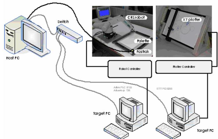
Figure 3 System Architecture
