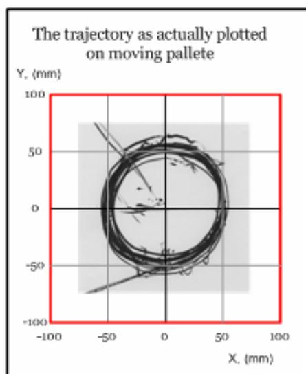
Figure 8 The tip's trace on the movable pallette
