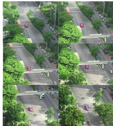
Fig. 9 Tracking the car, using the controller with image tracking.
