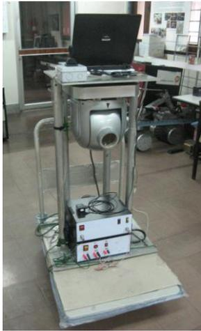
Fig. 10 The gimbal mounted on the mobile platform
