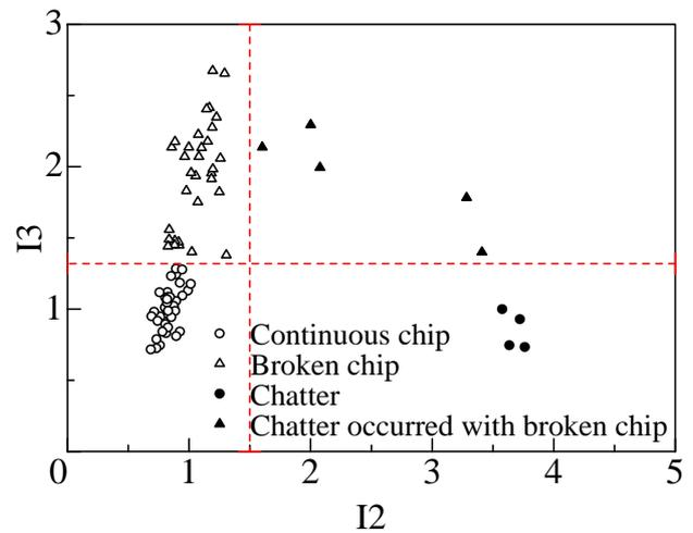
Figure 7. Illustration of the experimentally obtained reference feature space between I2 and I3.
