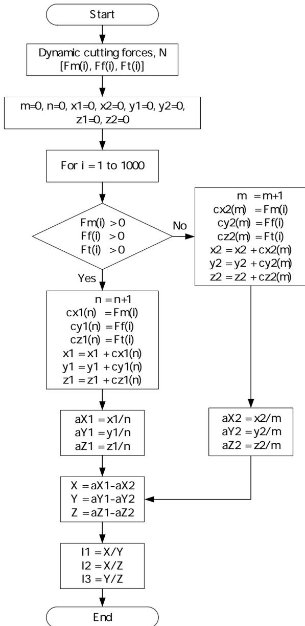
Figure 2. Flow chart of the algorithm to calculate the parameters I1, I2, and I3.
