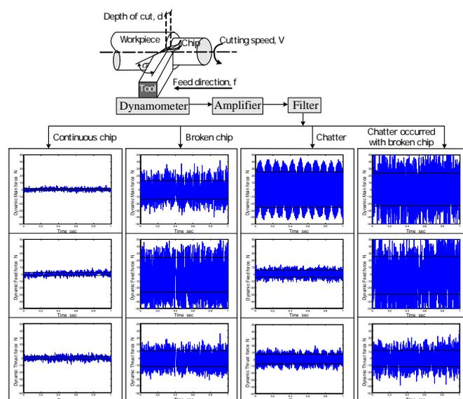
Figure 4. Illustration of typical examples of experimentally obtained dynamic cutting forces occurred at different cutting states.
