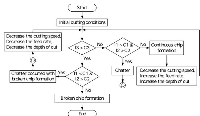
Figure 9. Flow chart of the algorithm to identify the states of cutting.
