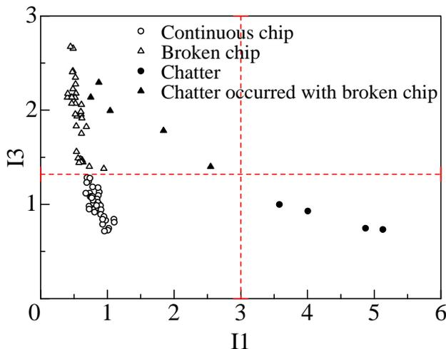
Figure 6. Illustration of the experimentally obtained reference feature space between I1 and I3.
