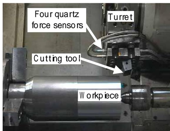
(b) New tool dynamometer installed onto tool turret of CNC turning machine.
