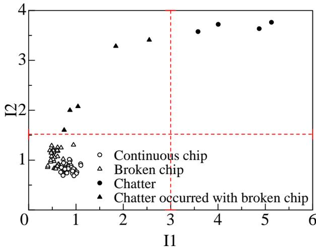
Figure 5. Illustration of the experimentally obtained reference feature space between I1 and I2.
