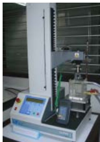
Fig 3 Nexygen from Lloyd Instrument Ltd with water bath for thermal control and thermocoupling to monitor temperature change.
