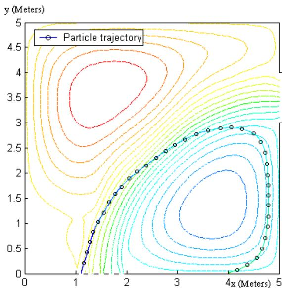
Figure 3: Stream function and particle trajectory of 30-micron-diameter particle with inlet grid.
