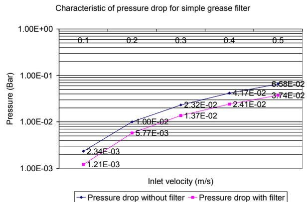
Figure 5 : The characteristic of pressure drop for simple grease filter
