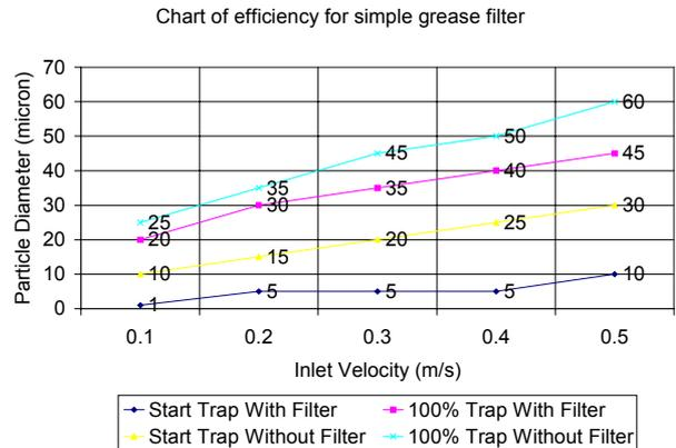
Figure 4: Chart of efficiency for filter with and without inlet-grid
