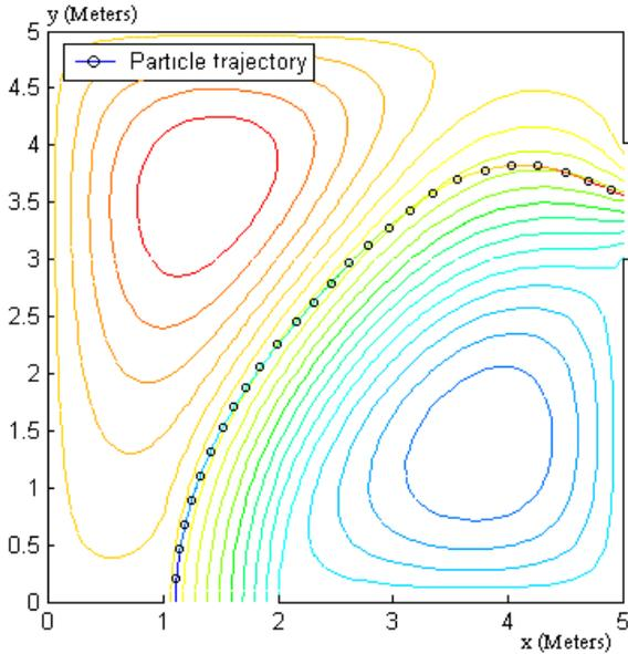
Figure 2: Stream function and particle trajectory of 30 micron-diameter particle without inlet grid.
