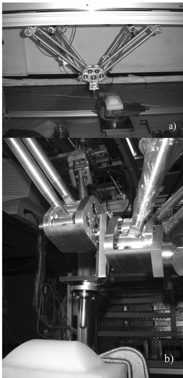
Figure 5 a) Prototyped new H-4 family parallel manipulator and b) Detail of moving platform and ATI mini45 force transducer of the prototyped new H4 family Manipulator
