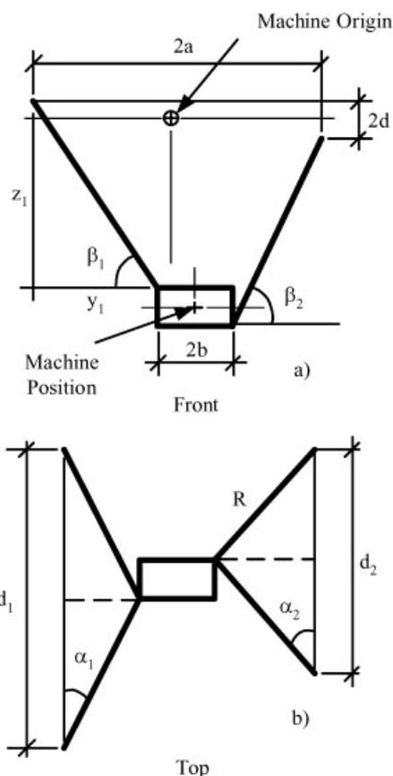
Figure 4 Position of manipulator viewing from the front and top represented by angle  $\alpha_1$   $\alpha_2$   $\beta_1$  and  $\beta_2$
