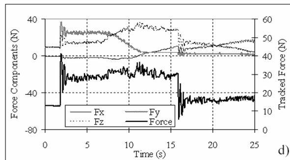
**Figure 6** a) Force tracking direction on resin surface b) Force tracking control on resin at 30 N and track speed at 21 cm/min. c) Force tracking control on resin at 20 N and track speed at 15 cm/min. and d) Force tracking control on resin with force step input changed from 30 to 15 N and tracking speed of 21 cm/min
