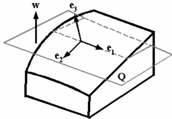
Figure 2 Determining Tracking direction in desired tracking plane from measured force
