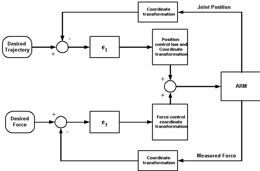
Figure 3 Implicit force control scheme used on prototype manipulator
