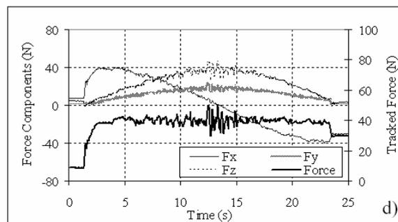
**Figure 7** a) Tracking direction on metallic surface b) Force tracking control on metal at 20 N and track speed at 21 cm/min c) Force tracking control on metal at 30 N and track speed at 21 cm/min and d) Force tracking control on Aluminum at 40 N and track speed at 60 cm/min
