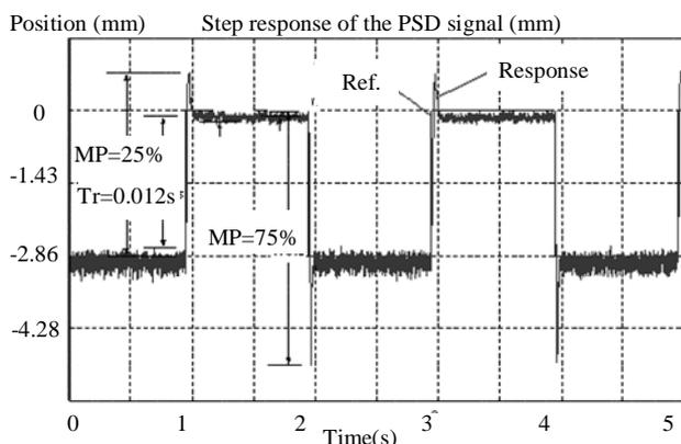
Figure 5, Step response of the PSD signal.
