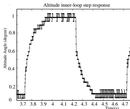
Figure 7, Step response of the altitude inner-loop.
