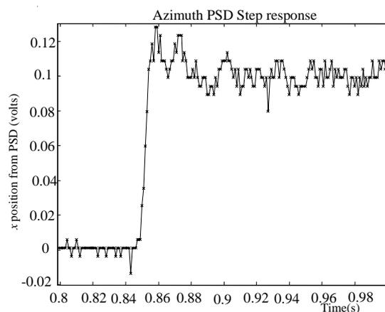
Figure 8, Step response of the azimuth PSD voltage.
