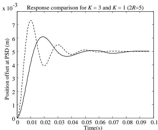
Figure 16, PSD Response for  $K = 3$  and  $K = 1$  ( $R=5$ )
