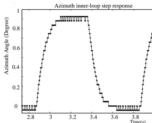
Figure 6, Step response of the azimuth inner-loop.
