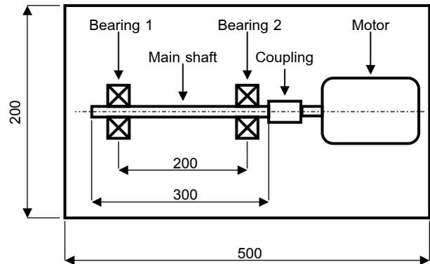
Fig.1: Schematic of the test rig, top view with sectioned bearings and overall dimensions (mm).
