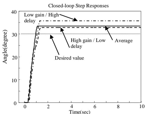
Figure 11, Step response of three subjects with a PD controller
