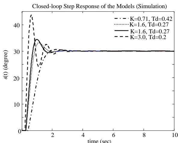
Figure 7, Closed-loop step response of human models with a P controller
