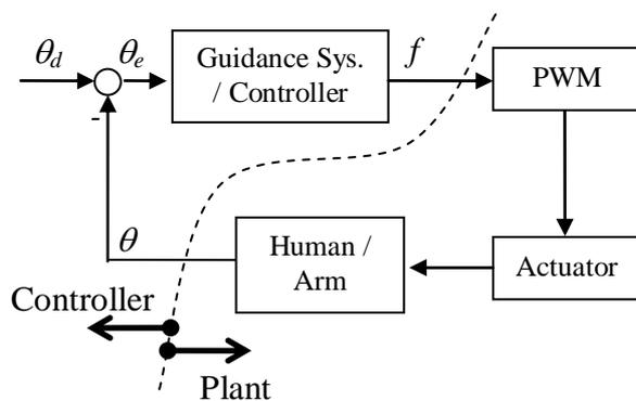
Figure 2, Vibrotactile guidance system schematics
