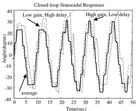
Figure 12, Sinusoidal response of three subjects with a PD controller
