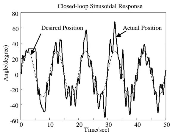
Figure 10, Sinusoidal responses of the subject #10 with a PID controller
