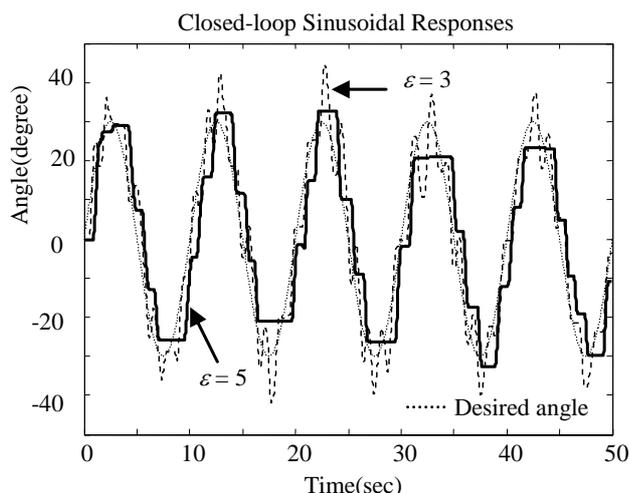
Figure 8, Closed-loop sinusoidal response of a subject #10 with on-off controller
