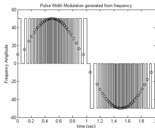
Figure 4, PWM signal generated from a sinusoid command  $f$
