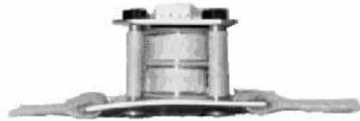
Figure 3, The vibrotactile signal generator (actuator)
