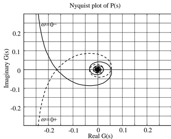
Figure 6, Nyquist plot of the transfer function  $P(s)$  with  $K = 1.6$  and  $T = 2.6$ .
