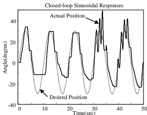
Figure 9, Closed-loop sinusoidal response of a subject #4 with the on-off controller ( $\epsilon = 5$ )
