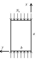
Fig. 4 A rectangular plate subjected to a uniaxial in-plane load
