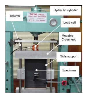
Fig. 1 The compression test frame for buckling experiment
