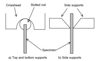
Fig. 2 The schematic of simply supported boundary condition
