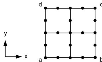
Figure 2 BE and FE mesh for the square plate (8 boundary elements and 4 cells).
