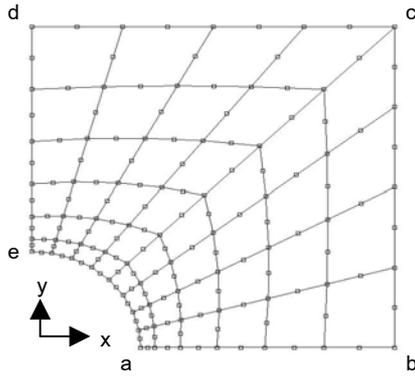
Figure 9 BE and FE mesh for the square plate with a circular hole (28 boundary elements and 48 cells).
