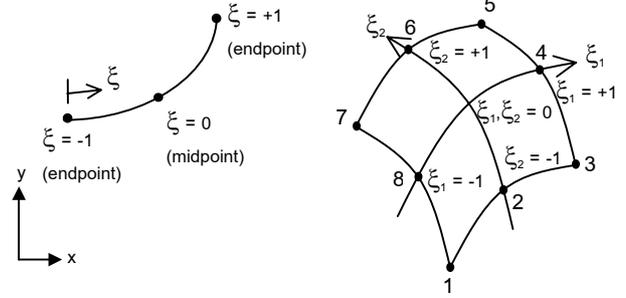
Figure 1 Isoparametric quadratic boundary element and cell.
