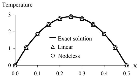
Figure 10 Temperature distribution along x axis at y = 0.5 of rectangular plate with sinusoidal temperature at top edge and internal heat generation.
