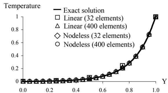
Figure 6 Temperature distribution along y axis at  $x = 0.25$
