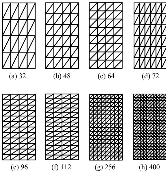
Figure 4. Finite element number of rectangular plate.
