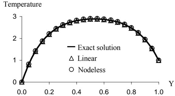
Figure 11 Temperature distribution along y axis at x = 0.25 of rectangular plate with sinusoidal temperature at top edge and internal heat generation.
