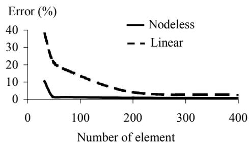
Figure 8 Error of temperature along y axis at  $x = 0.25$
