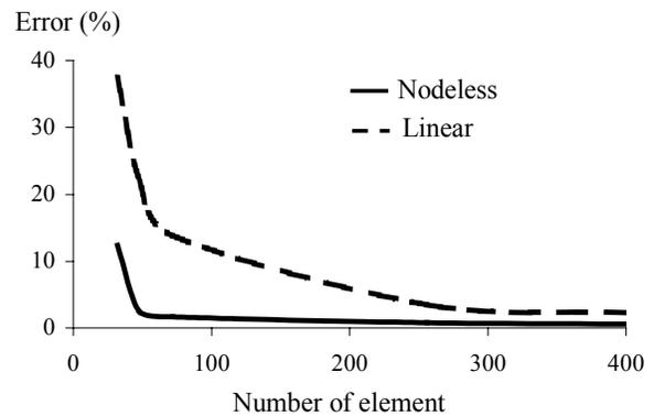
Figure 7 Error of temperature along x axis at  $y = 0.5$
