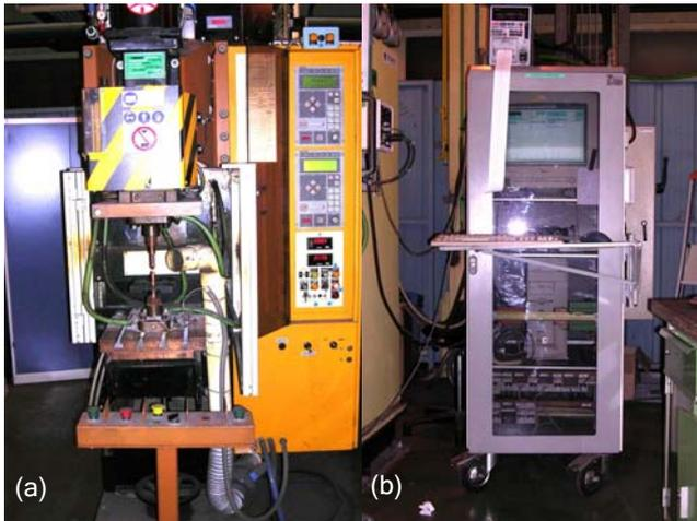
**Fig. 1:** Experiment facility used conducting the welding experiments; (a) Pedestal resistance spot welding machine, and (b) Signal monitoring and acquisition setup
