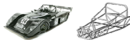
Figure 6. Example of a spaceframe chassis from Juno Racing Ltd. [5].
