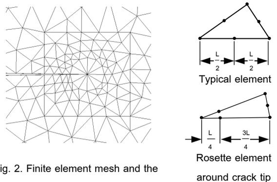
Fig. 2. Finite element mesh and the elements used on integrated domain
